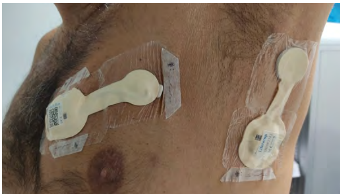
Figure 2 On the left, the Lifetouch Blue sensor (electrocardiographic monitoring). On the right, the Lifetemp Sensor (temperature monitoring).
