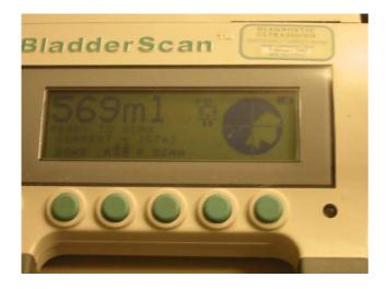
Fig. 4. BladderScan<sup>TM</sup> BVI 3000. Close up of the screen. The volume bladder is shown on the left and the icon on the right demonstrates a good quality scan because the white area extends across the crosshairs of the dark circle.
